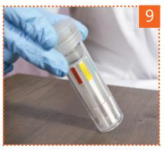
Sometimes, especially when the sample isn't homogenized, liquid migration can stop on one or more strips. In that case, tap the end of the strip tube on hard surface to allow migration to start again.
