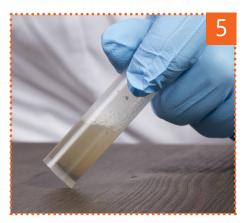
■ Tap the sample tube on a hard surface so that all the liquid is collected at the bottom of the tube.
