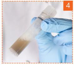
■ Shake the sample tube to homogenize well.
