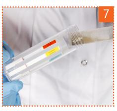
Insert the sample tube into the strip tube.
